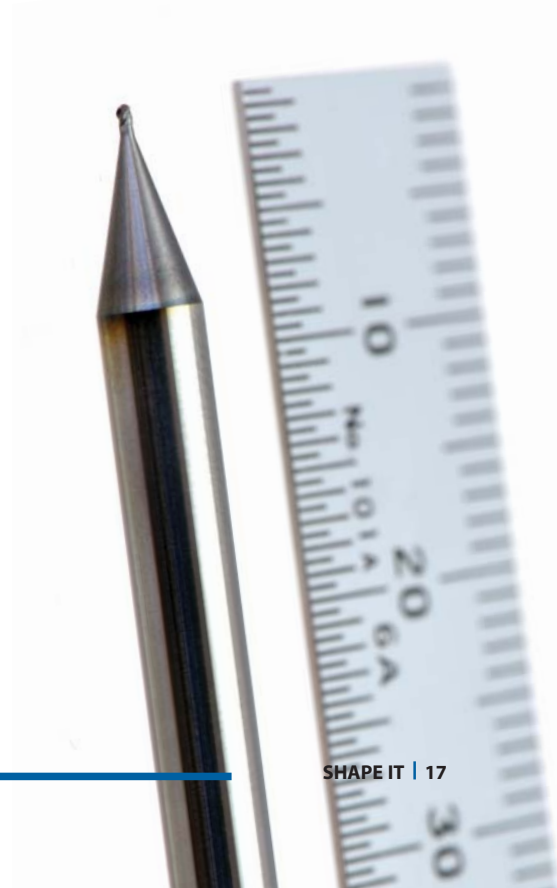
Thanks to its unique 3-flute geometry, the PHX-LN-DBT can serve as a finishing tool. Further, the PHX-LN-DBT's strong helix angle ensures that the tool exhibits very low radial deviation to accommodate tight tolerance requirement.
