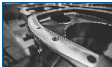
Top: Prior to the XPF forming tap, Valtra was using a cut tap to thread their fuel tanks in SAE 1020 steel and was troubled by bird nesting problems.
